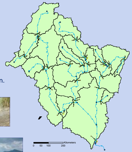
Figure 4: Set up of the network model Mike Basin for the Volta basin integrating different water users per subcatchment.
